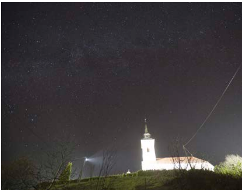
A shielded luminaire with an MH bulb with 3000 K and additional filter that blocks UV and blue light.
