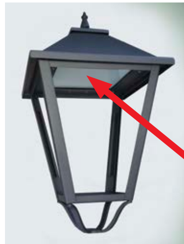
An example of a stylish lamp for the illumination of the vicinity of objects of cultural heritage. The bulb is placed in the upper part. The luminaire has no side glasses since these scatter light above the horizontal.
