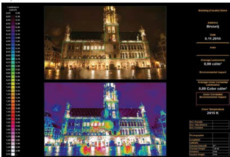
City Hall at the Grand Place in Brussels. Despite the fact that Belgium is the most light-polluted country in the EU, the façade luminance of the greater part of this side of the building (without illuminated windows and lamps) is under 1 cd/m 2 .
